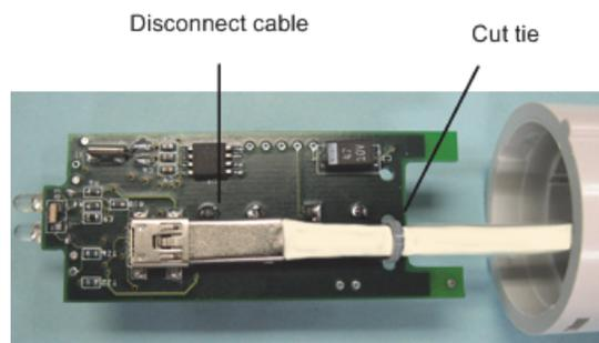
7. Pull the cable out through the case.
