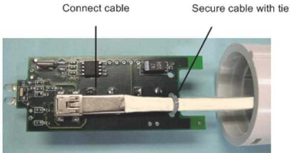
4. Secure the cable to the board using the cable tie (included). Feed the tie through the two holes near the end of the board, with the cable tie's 'buckle' on the battery side of the board. Ensure that cable tie is tight and then trim the end.
