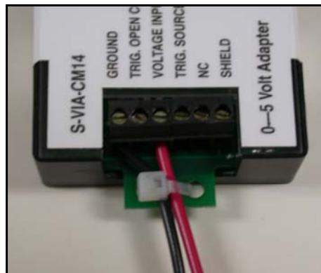
Figure 1: Cable strain relief
