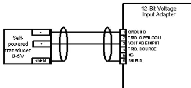
Figure 2: Transducer setup
